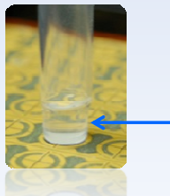
Figure 2. Lambda DNA sample, as indicated by the blue arrow in the figure, in an off-the-shelf Matrix 2D-barcoded storage tube is positioned over a BLU energy form factor to be sheared to target fragment length.
