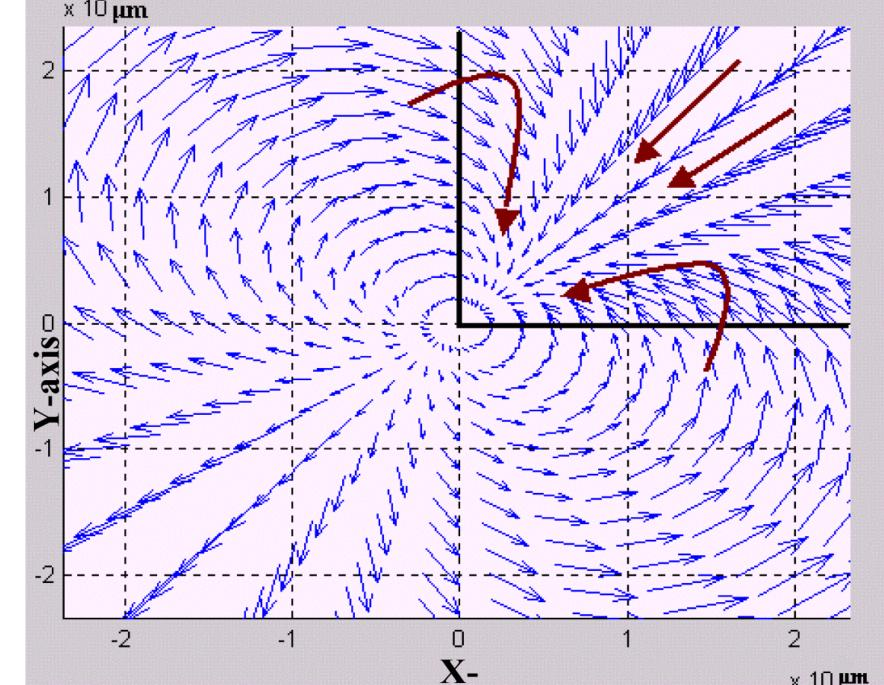
Fig. 3 Simulated vector field of particle displacements at a plane above the micromixer cell.
