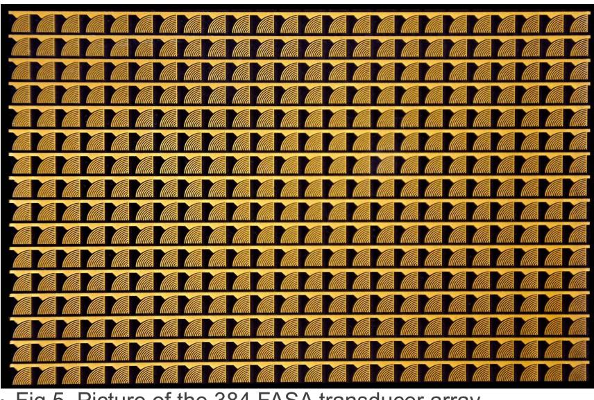
• Fig 5. Picture of the 384 FASA transducer array
