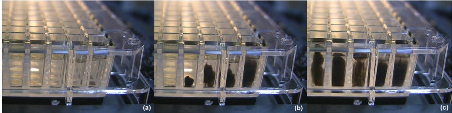
Fig 9. Shows mixing and resuspension of beads in water. (a) 0 sec. (b) 5 sec. (c) 10 sec.
