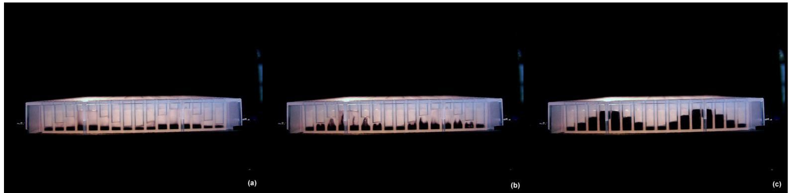
Fig 7. Shows mixing of dye in water. (a) 0 sec. (b) 5 sec. (c) 10 sec.
