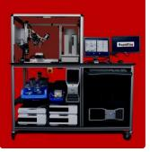
We compared the results of various HENDRIX SM100 settings to determine the optimal operating conditions and achieved a 50% improvement in the triolein signal-to-noise ratio in the RF-MS assay.
